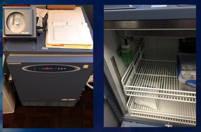
Helmer Blood Refrigerator, multiple thermometers and alarms, including cellular connectivity. Keeps blood between 3-5 degrees Celsius
